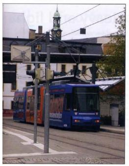
three-rail track, has a length of about 1100 m. The distances between the track centres of the metre gauge tramway are 3.9 m, for the standard gauge railway tracks it is 3.47 m. Trams are 2.3 m wide, the *Regiosprinter* 2.97 m. It is still possible to use the tracks with replacement buses or emergency vehicles.
